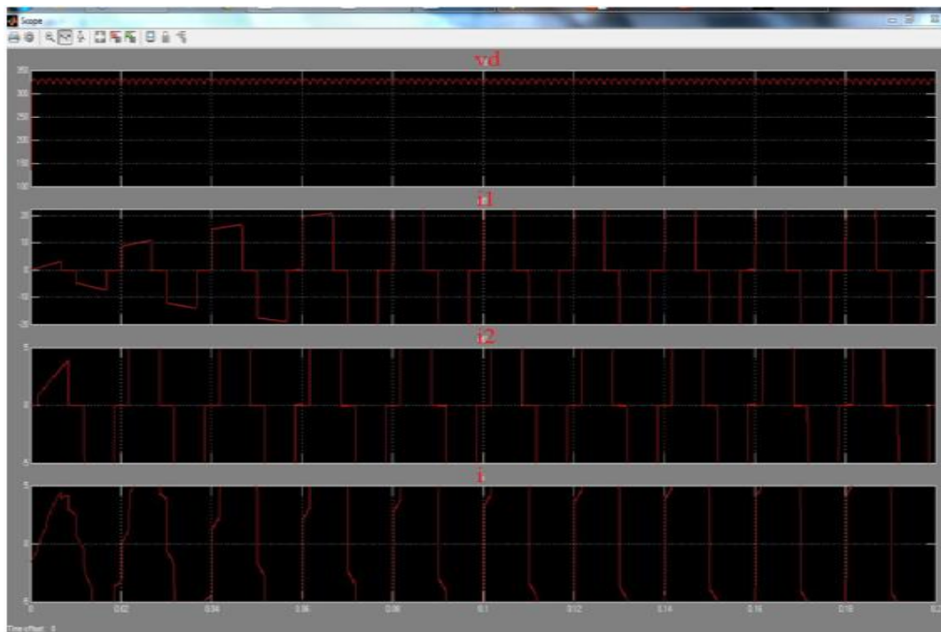
Figure: 5: waveforms of twelve pulse converter using diodes.
