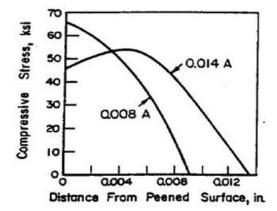
The test sections of the specimens were hand polished in the longitudinal direction with 180- grit emery paper, shot peened and subjected to axial fatigue loading.
