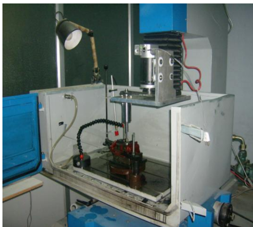
Fig. 3 Photograph of assembled setup on ZNC EDM machine
