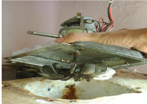
Figure 1: Profile of Pyro Hydro Turbine
