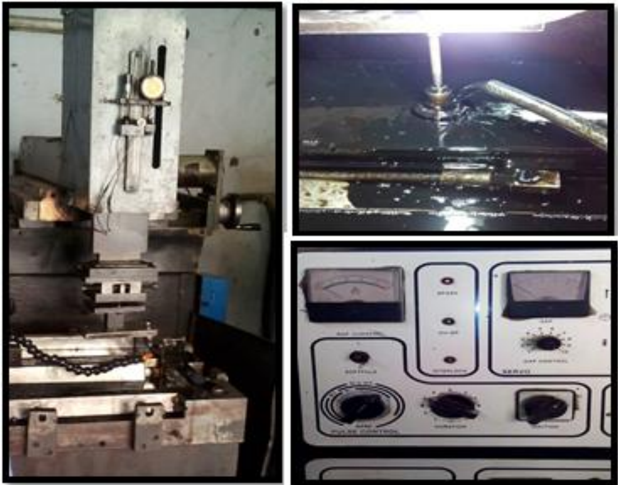
Figure 2: EDM Machine and Control Panel
