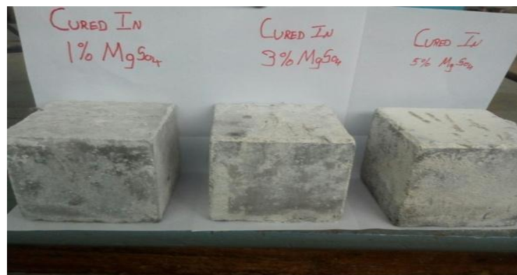
Fig.3 Cubes cured in different percentages of MgSO 4
