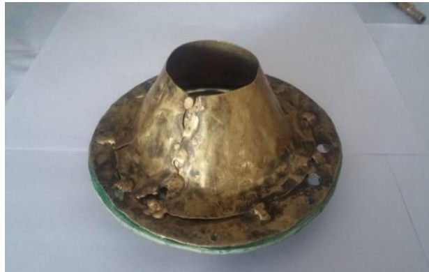
Fig.12 Exhaust cone with heat resistant gasket
