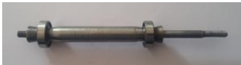
Fig.5 Shaft with bearings and spacers
