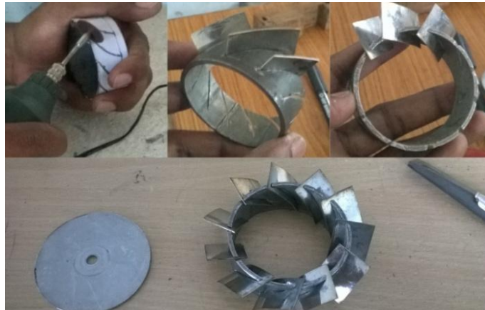
Fig.10 Nozzle guide vanes system machining
