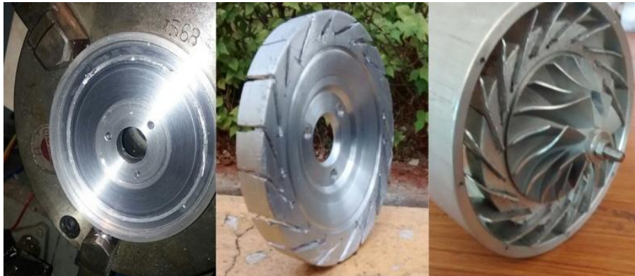
Fig.4 Compressor guide vane system machining
