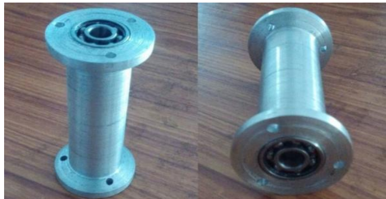
Fig.6 Shaft tunnel with bearings
