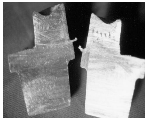
Fig.8: Section of casting with Insulated Riser of H/D=1
