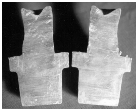
Fig.7: Section of casting with insulated Riser
