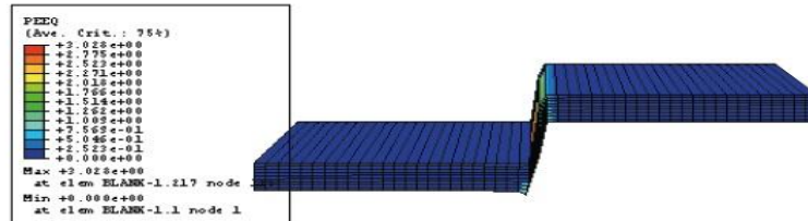
Fig. 4: Contour of shape after blanking process of mild steel 2 mm.
