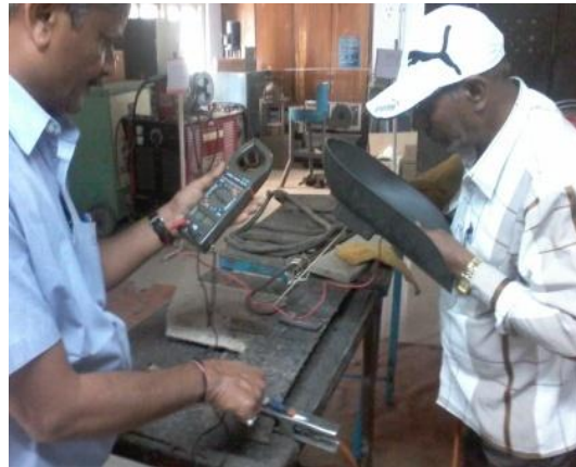
Fig-7 Measurement of arc voltage using multimeter
