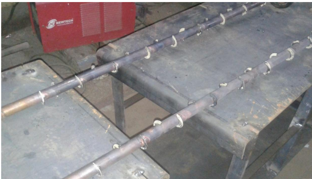
Figure 2: Inner tube having semi-circular fins
