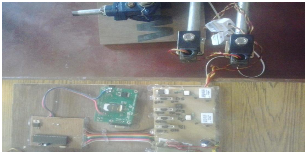
Fig.7.1. Complete Assembly of Microcontroller based Automatic Sprinkler System
