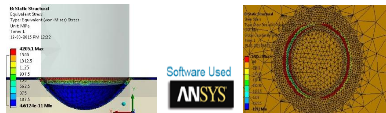
Fig.5 FEA Results for EQV and Shear Stress (Assembly Model-C)
