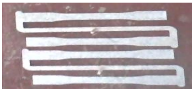
Fig.2 Tensile test specimens produced by injection moulding machine.
