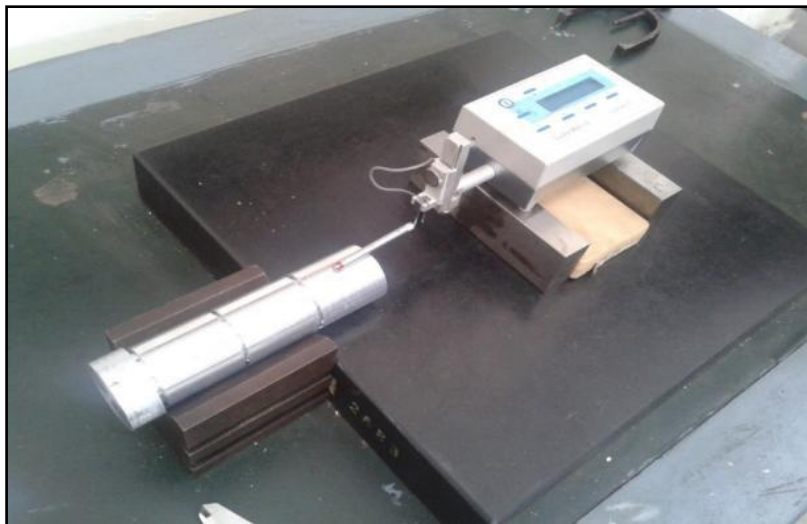
Fig. 2: Roughness Measuring Instrument(Taylor Hobson Surtronic 3+)
