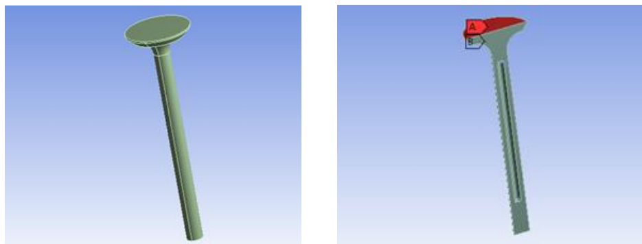
Fig. 3. CAD Model of valve with and without air cavity
