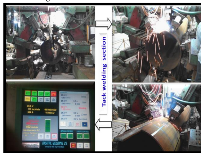
Figure 3: GMAW auto tack welding
