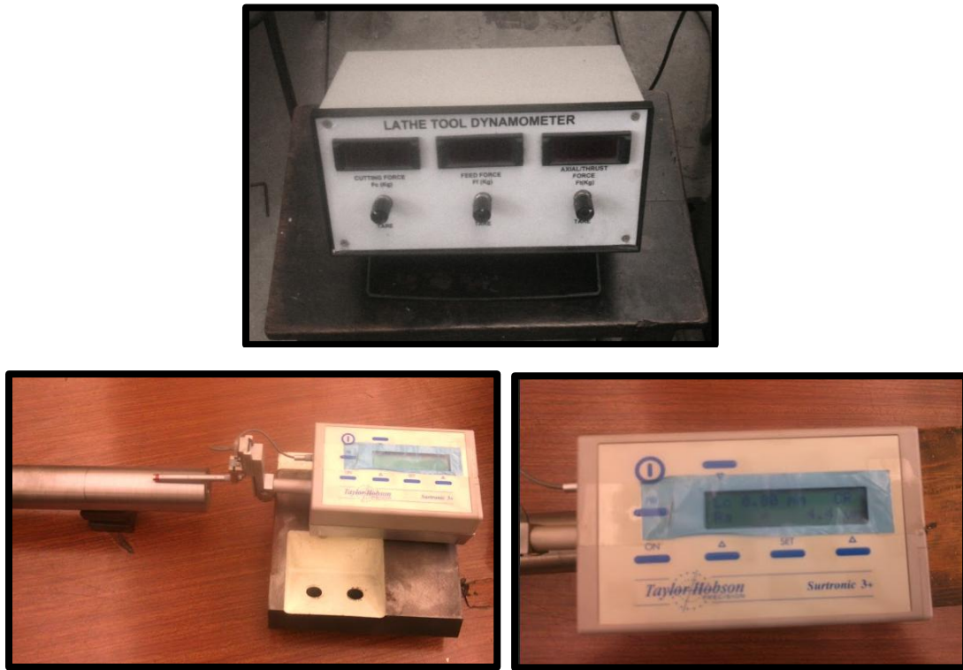
Fig. 2: Lathe tool dynamometer (top) and Surtronic 3+, roughness testing machine in use
