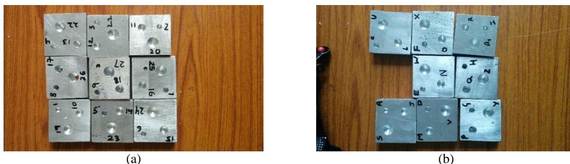
Figure 2: Photographic View of Al-B 4 C p Drilled pieces
