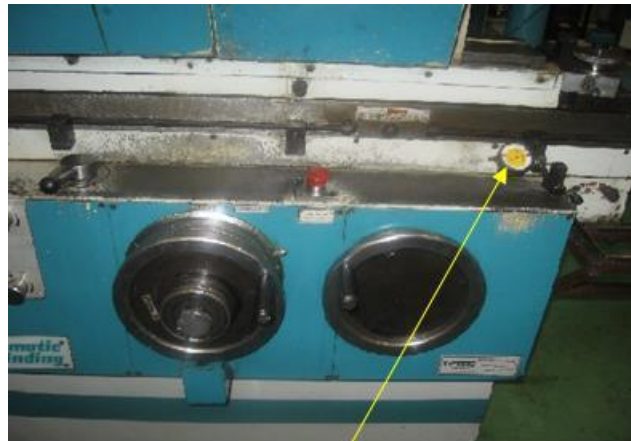
Dial provided on grinding machine slide , to set the proper location of grinding wheel after the wheel dressing.
