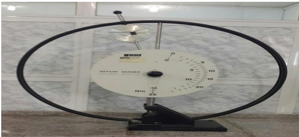
Figure (3): Impact test instrument.
