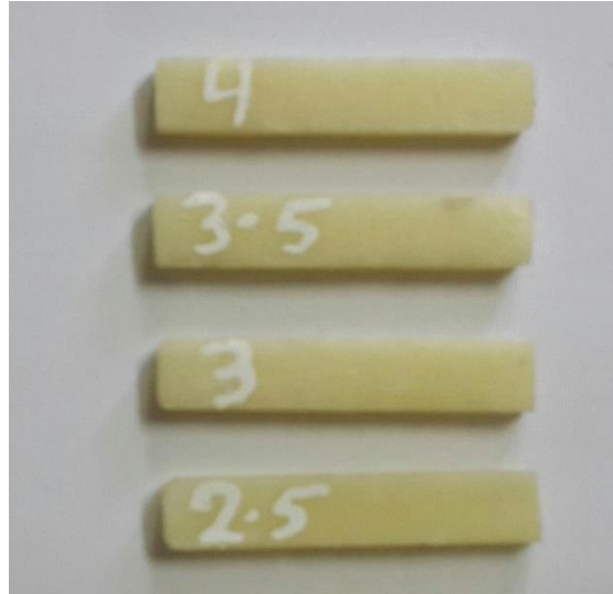
Figure (2): the standard specimen according to ISO-179.
