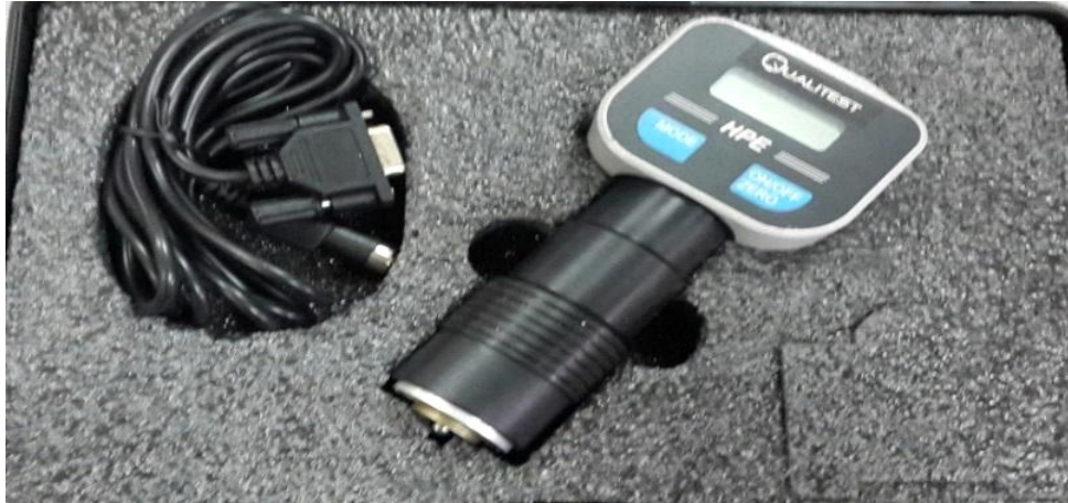
Figure (1): The digital durometer pocket size model for shore D hardness testing "Digitat hand-held hardness tester".
