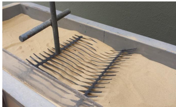
Figure 16b: Geogrid preparation ( L/B=2.5 )
