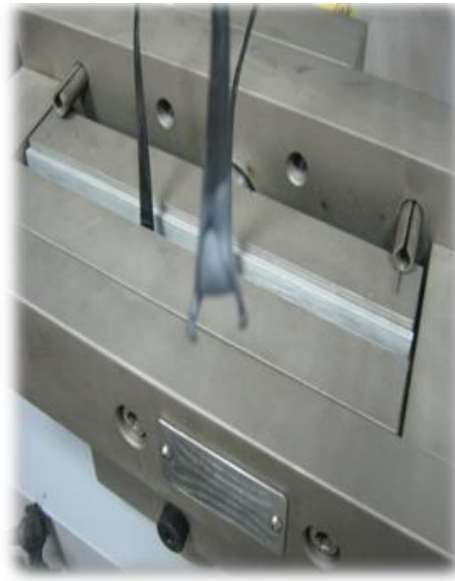
Figure 6: Geogrid Junction Rupture
