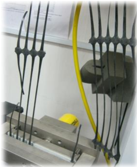
Figure 6: Geogrid Junction Rupture
