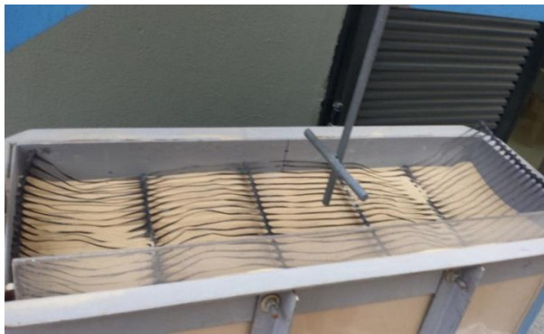
Figure 16a: Geogrid preparation ( L/B=12 )
