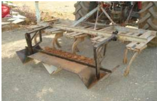
Fig. 5 Raised bed preparator attached with cultivator
