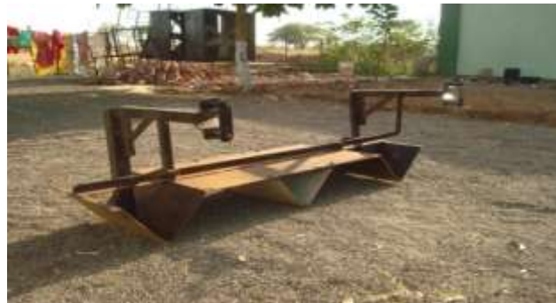
Fig.4 Raised bed preparator frame
