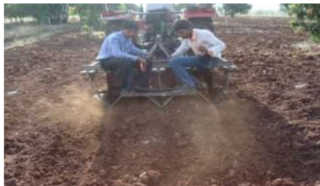
Fig.6 Actual working of the raised bed preparator in field
