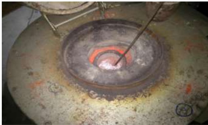
Figure 2.1 Pot furnace, with a stirrer
