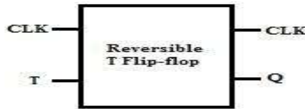
Figure . 8 Block Diagram of Reversible T flip-flop
