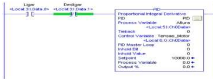
Figure 4: PID Controller Embedded on the Plant's PLC.
