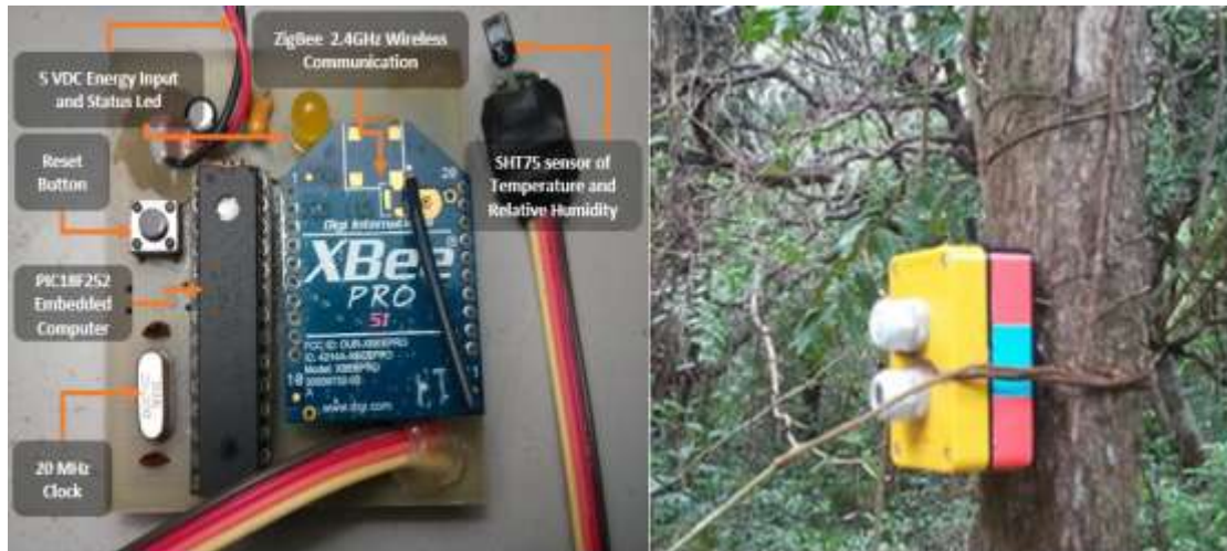
Fig 1 Sensory platform architecture fixed to a tree, in a height of 1.5 meters from the floor.
