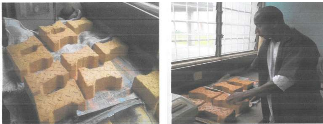
Fig. 2: Interlocking blocks made from locally fabricated moulds
