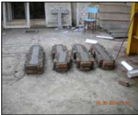
Fig.5 Casting of specimens
