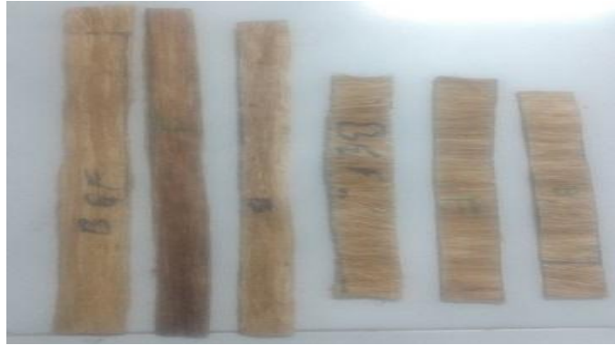
Three Tensile Testing Samples are cut in both X and Y- direction
