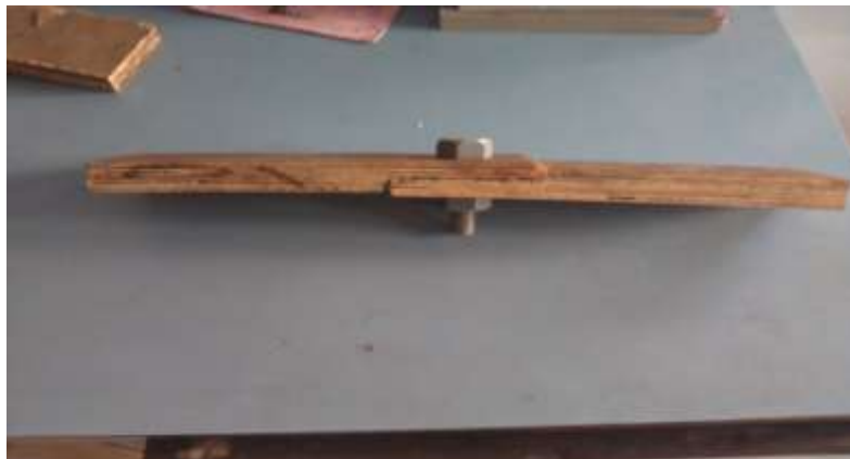
Fig 18: Wood work pieces joint with bolt and nut
