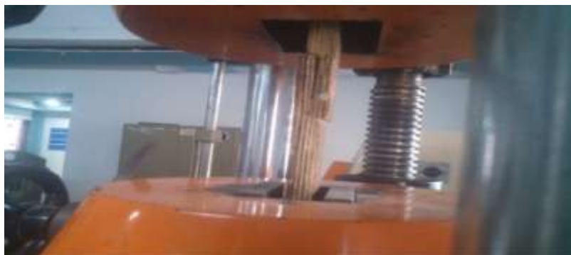
Fig 19: Wood work pieces joint with bolt and nut in UTM
