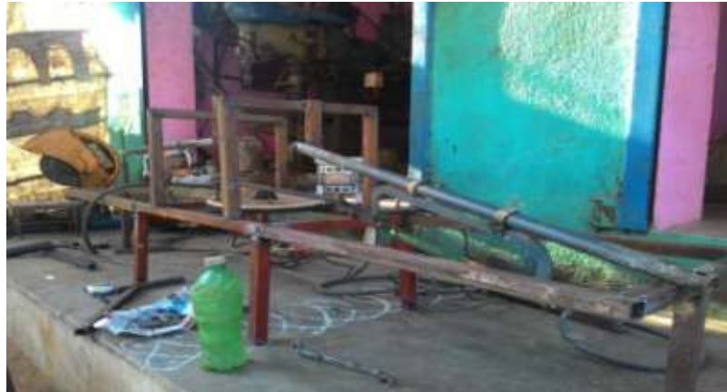
Fig 3.2.5 Main frame attached with two side frames
