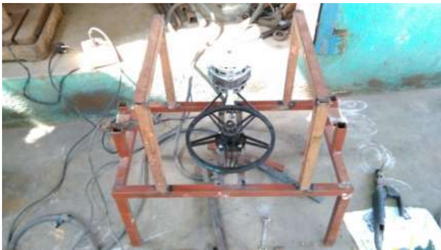
Fig 3.2.3 Motor with pulley in main frame
