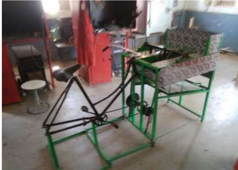
Fig 3: Actual model of pedal operated groundnut decorticator machine
