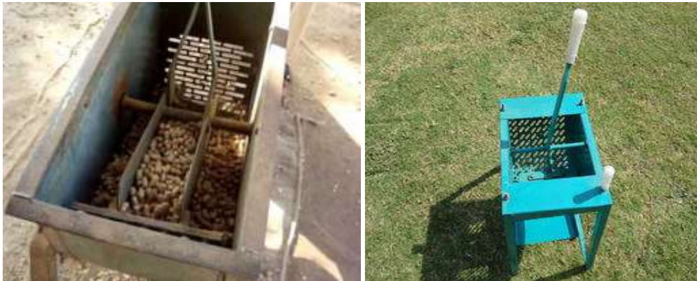
Fig 4: Actual model of hand operated groundnut decorticator [7]
