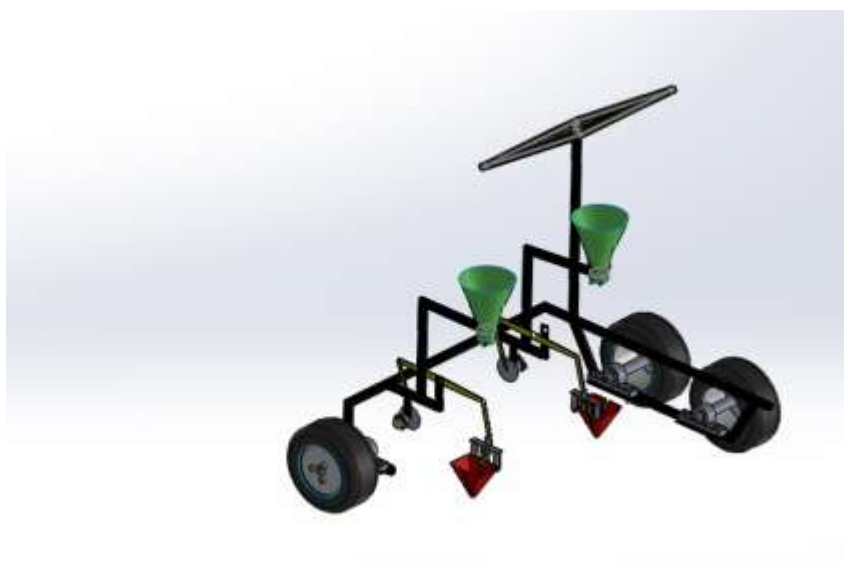
Fig 2.1 Developed Vegetable planter machine
