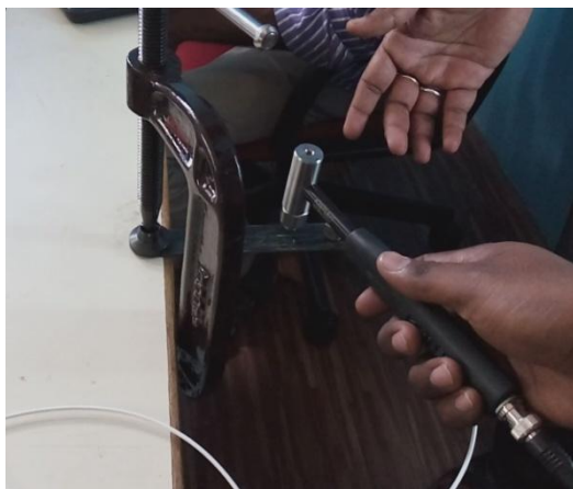
Figure 5: Excitation given by Impact Hammer Figure 6: Vibration analysis by FFT analyzer
