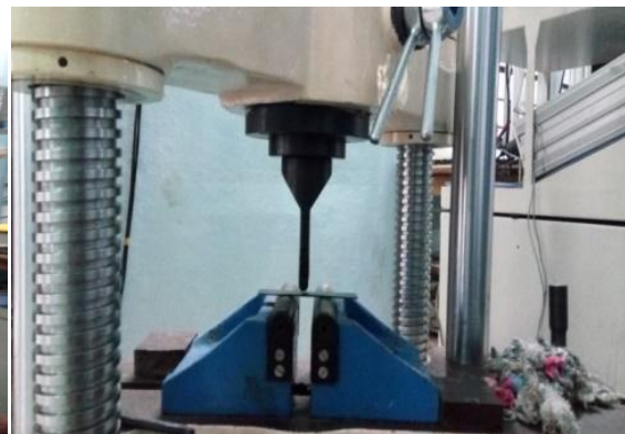
Figure 3: Tensile Test by using UTM Figure 4: Flexural Test by Using UTM
