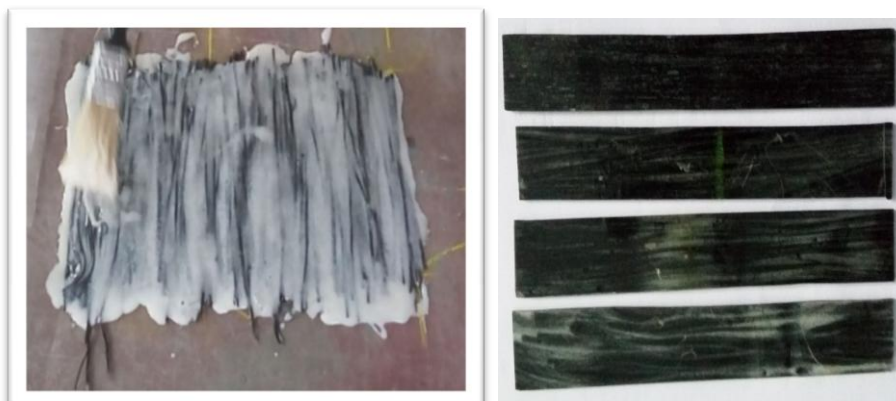
Figure1: Fabrication of Composite Beams Figure2: Prepared Composite Beams
