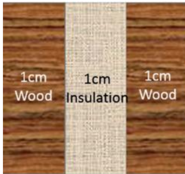
Fig: 7: Schematic of the wall showing the location of the insulating mats. [13]
