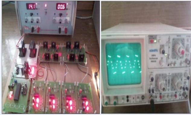
Fig.18. Experimental Arrangement of Neutral Clamped Multilevel Z-Source Inverter
