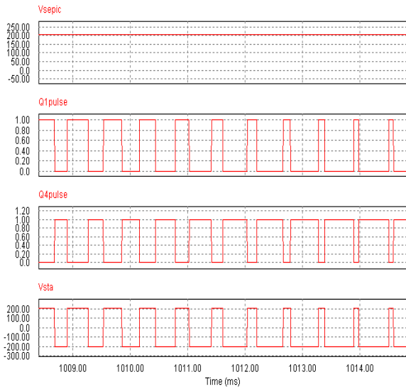
Fig. 8 The SEPIC converter output voltage and the inverted output voltage as a result of SPWM pulses
