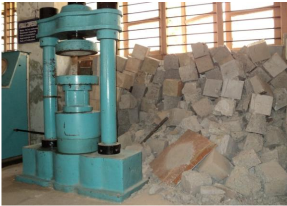
Fig 1. Section of tested cube specimens in Compression Testing Machine
