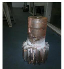
Figure3: Helical pinion of traction motor
