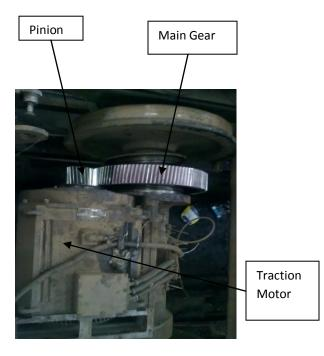
Figure 2 Traction motor asssembly
